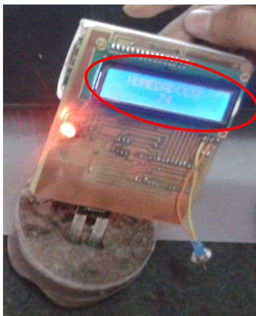
Figura 85. LCD sensor inalámbrico (emisor Rf).
