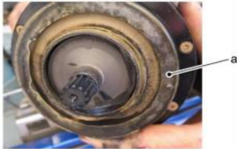
A OIL LEAK ON THE INTERFACE OF THE STARTER GENERATOR
