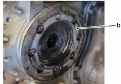
C OIL SEEPAGE
