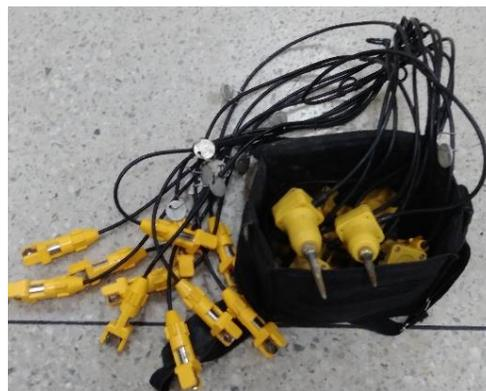
**Figura 72***Cable de extensión para el martillo*
