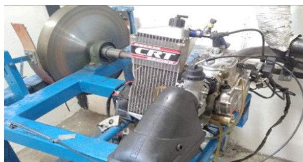
Figure 4 Rotax engine on the dynamometer.
