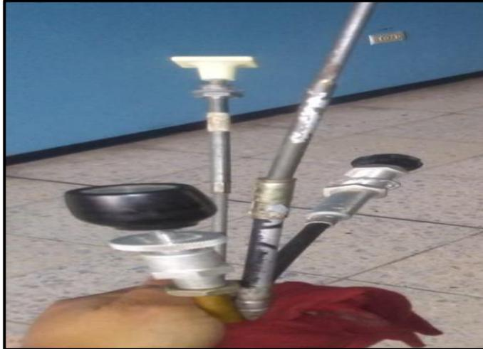
***Cables del mixture control and throttle***
