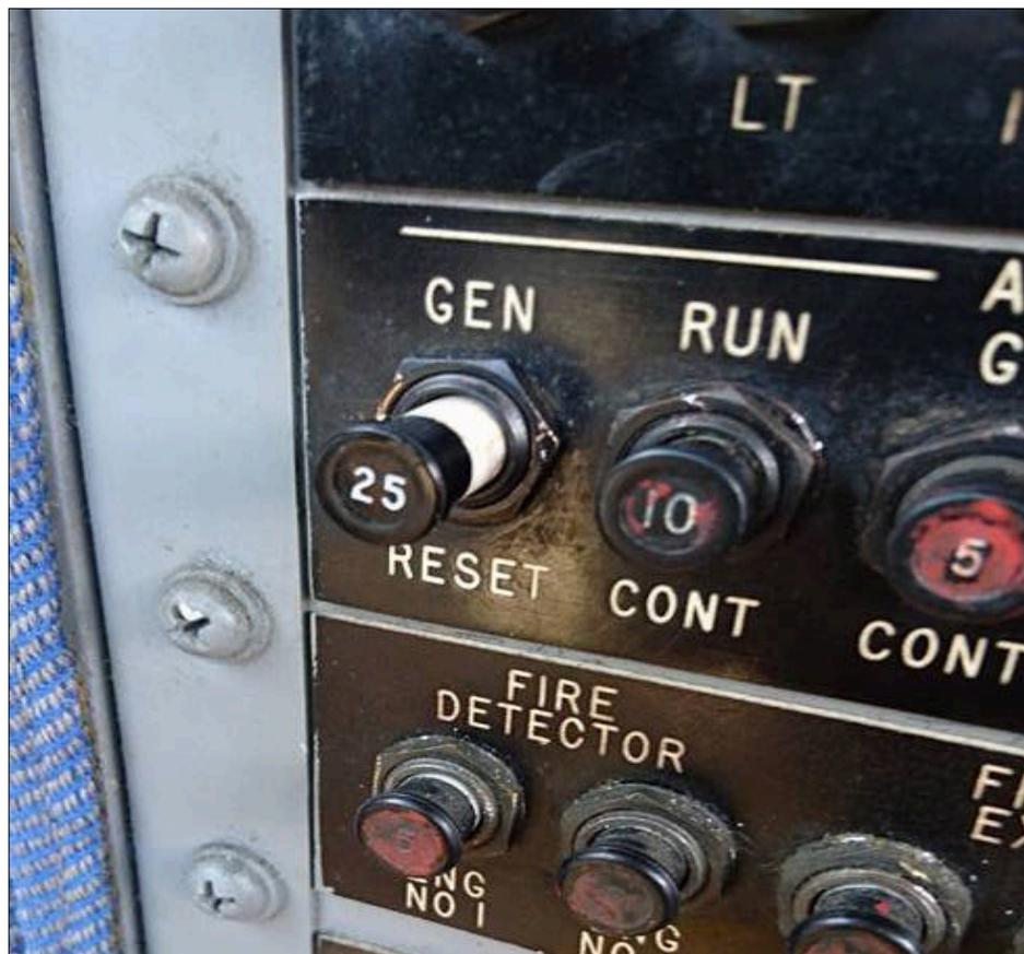
Figura 21 Circuitbreaker
