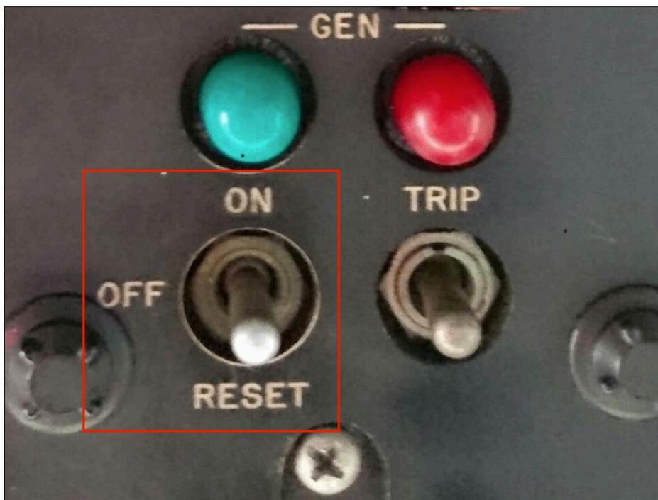
**Figura 7 Interruptor ON / OFF / RESET**
