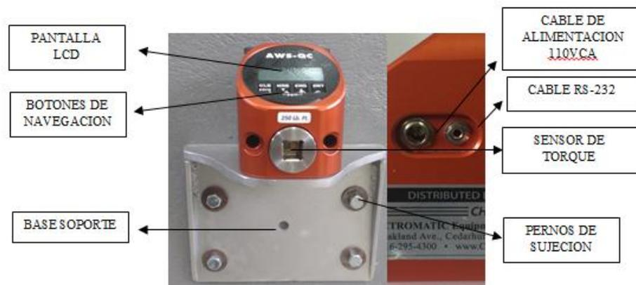
**Figura 68** AWS-QC Torque Tester
