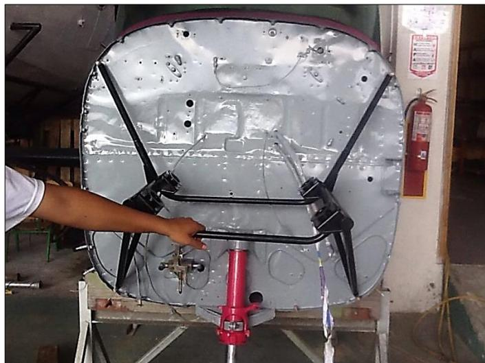
**Figura 26 Engine Mount Instalado**
