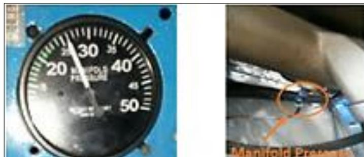
**Figura 50 Manifold Pressure**
