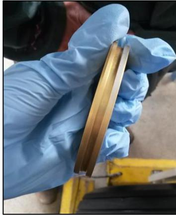
**Figura 112** Thrust Bearing
