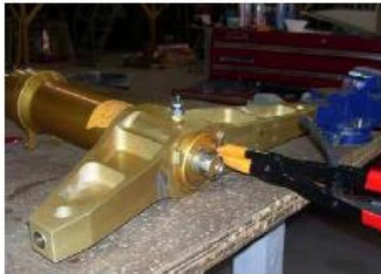
Figure 32-32 — Cylinder Tube Cap Retainer Snap Ring
