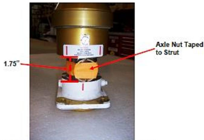
**Figure 5-14: Strut Compressed with Axle Nut Spacer**
