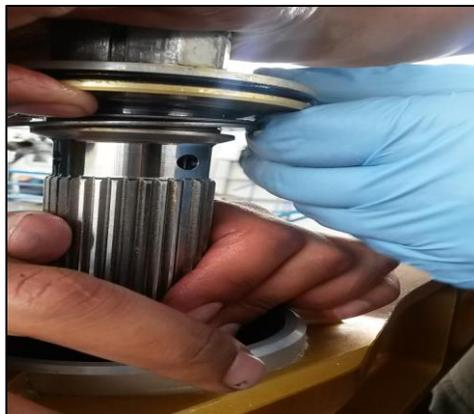
**Figura 107** Thrust Bearing Assembly y Outer Tube Cap
