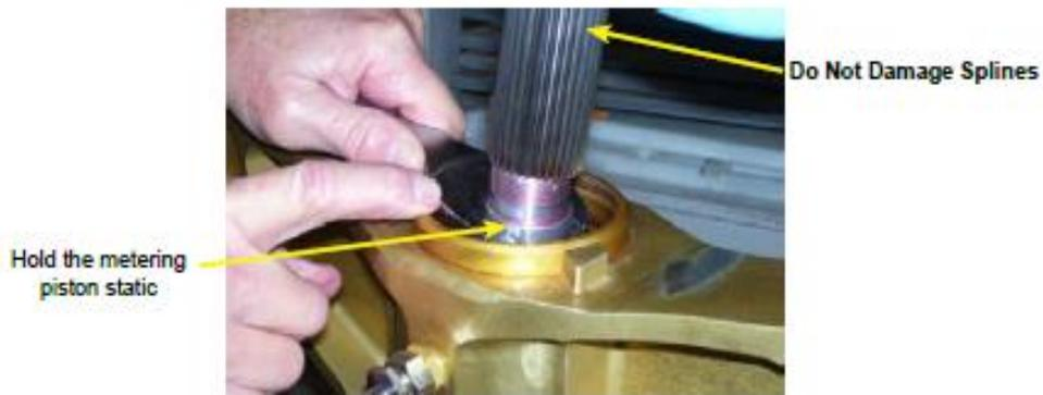
Figure 32-34 — Steering Tube Removed
