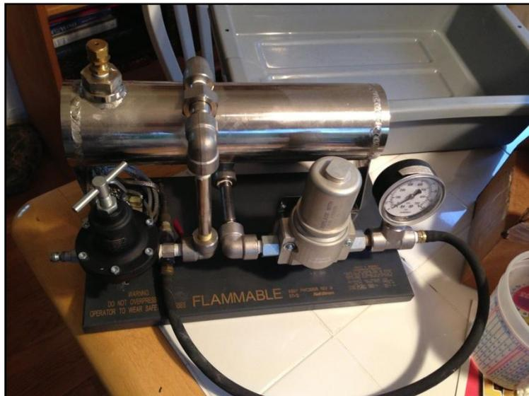
**Figura 3.1** Tester Fuel Nozzle.
