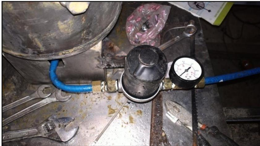
**Figura 3.5** Tester Fuel Nozzle.
