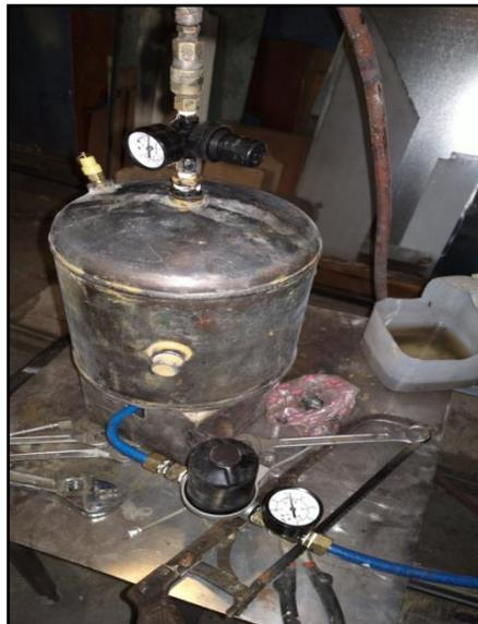
**Figura 3.2** Tester Fuel Nozzle.
