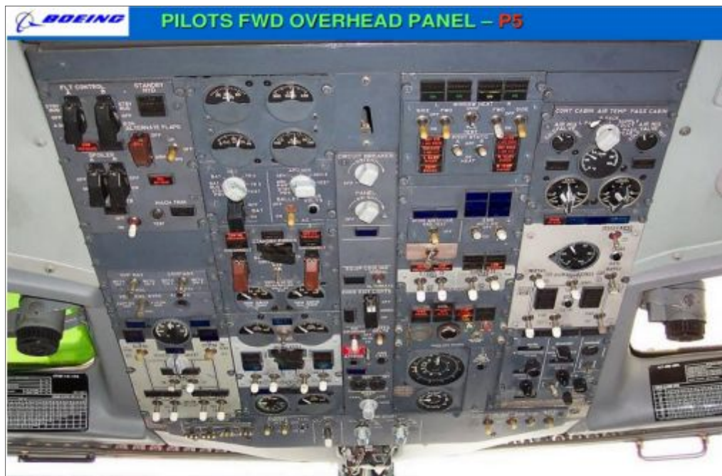
Figura 2. 25: Panel p5 del Boeing 737-200
