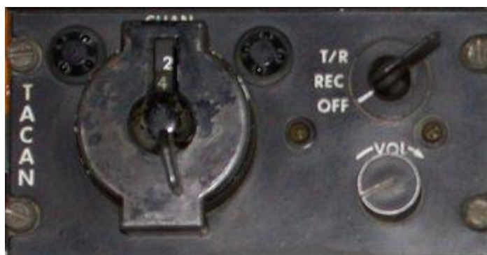
Figura 3.30 Panel de control TACAN
