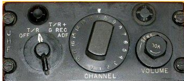
Figura 3.31 Panel de control UHF
