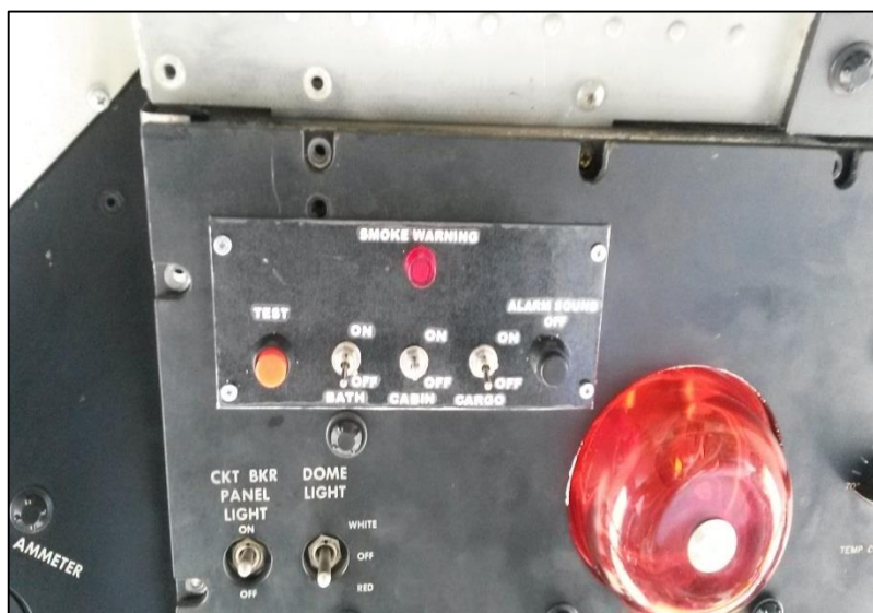
Figura 36: Panel smoke warning
