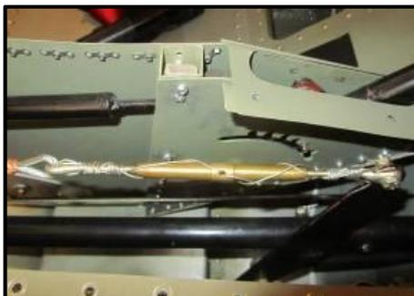
**Figura 46.** Turnbuckle
