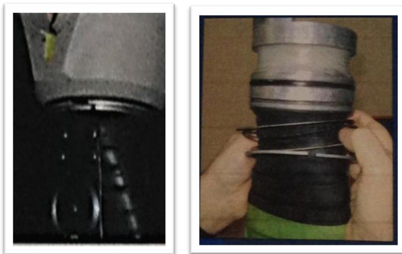
**Figuras 30:** Retaining ring, shims, shim carrier, thick shim
