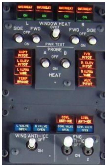
Figura N° 2.5: Boeing 737-NG Ice & Rain Panel
