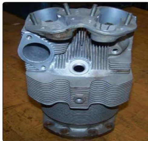
Figura 6 Cilindro del motor Fuente: (ADMINISTRATION, Aviation Maintenance Technician Handbook–Powerplant , 2012)
