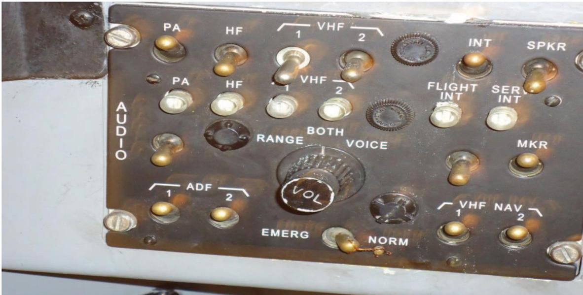
**Figura 3.14: Instrumento selector de audio**
