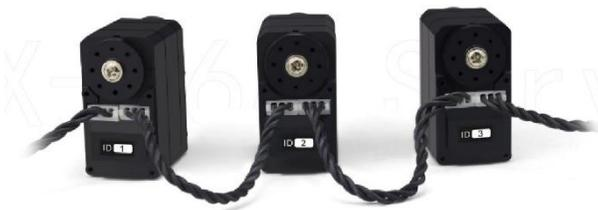
Nota. Tomado de *Hiwonder LX-16A Full Metal Gear Serial Bus Servo with Real-Time Feedback Function for RC Robot (Control Angle 240)* por Hiwonder, 2021 (<https://www.hiwonder.hk/products/hiwonder-lx-16a-full-metal-gear-serial-bus-servo>)
