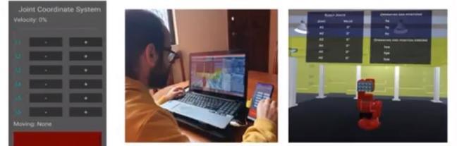
The interface shows a 'Joint Coordinate System Velocity: 0%' control panel with a 'DEADMAN SWITCH' button. On the right, a person is shown using a laptop and a smartphone to interact with a virtual environment where a robot arm is visible.
