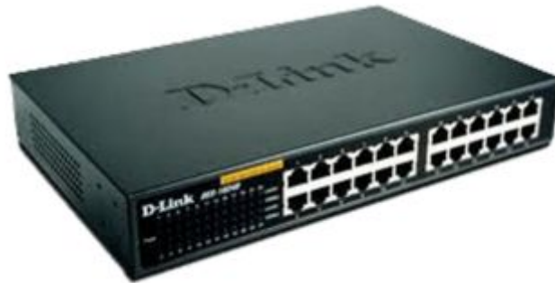
Figura 22. Switch D-link no administrable
