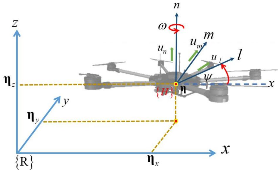
$$\begin{bmatrix} \dot{\eta}_x \\ \dot{\eta}_y \\ \dot{\eta}_z \\ \dot{\psi} \end{bmatrix} = \begin{bmatrix} \cos\psi & -\sin\psi & 0 & 0 \\ \sin\psi & \cos\psi & 0 & 0 \\ 0 & 0 & 1 & 0 \\ 0 & 0 & 0 & 1 \end{bmatrix} \begin{bmatrix} u_l \\ u_m \\ u_n \\ \omega \end{bmatrix}$$
