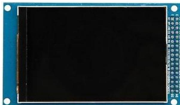
**Figura 2.22. TFT Shield Arduino**
