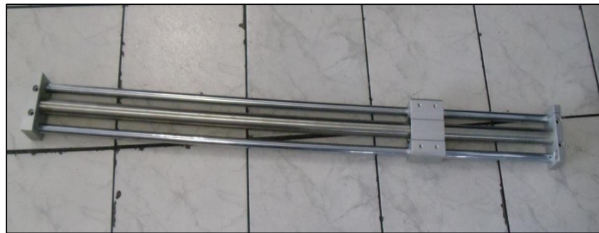
Figura No. 3.43: MRU 32x1200mm Marca Chelic
