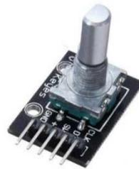
**Figura 29. Rotary Encoder**
