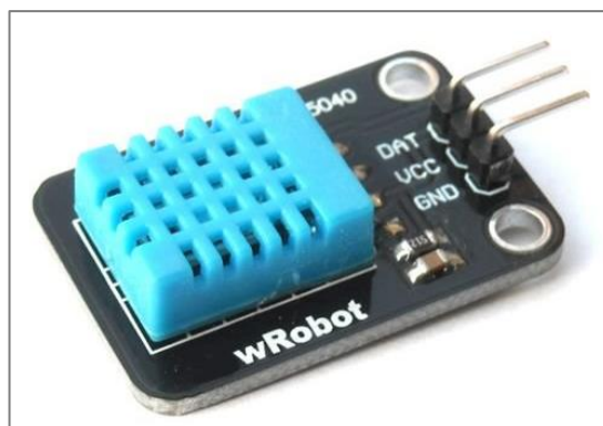
Figura 53. Sensor DHT11 Fuente (wRobot, 2014)
