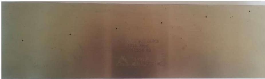
Figura 48 Bloque Navships Test Block Acero 1018
