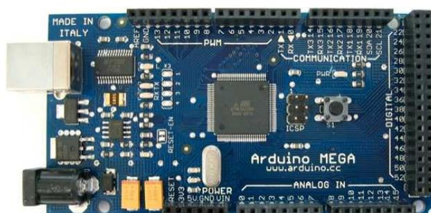
**Figura 2. 19 Arduino Mega 2560**
