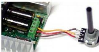
**Figura 100: Circuito de control del driver Sabertooth 2 X 25**
