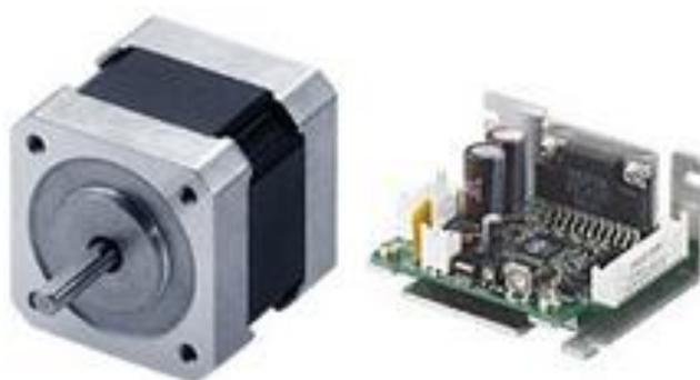
**Figura 14: Motor paso a paso.**
