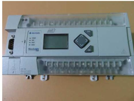
**Figura 49. PLC Micrologix 1400**
