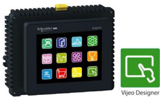
Figura 51. Touch Panel programado con Vijeo Designer. (Schneider Electric, 2011)
