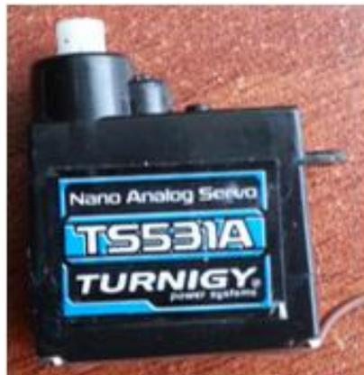
**Figura 138. Servomotor TURNIGY TS531A**
