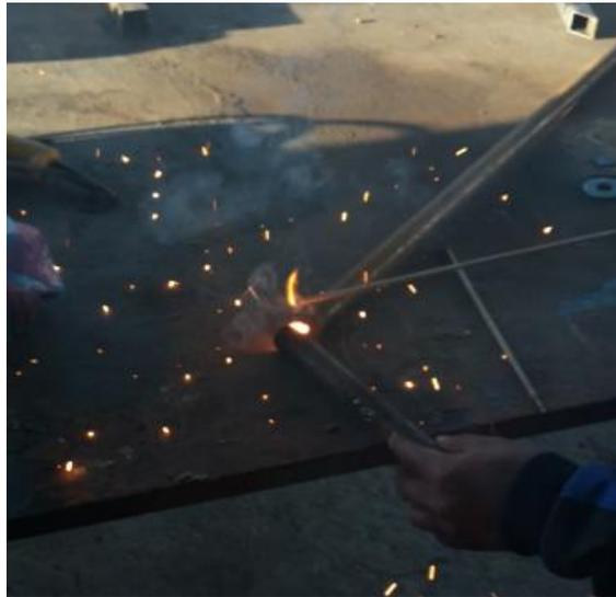
Figura 84 Unión de tubos redondos ASTM A36.
