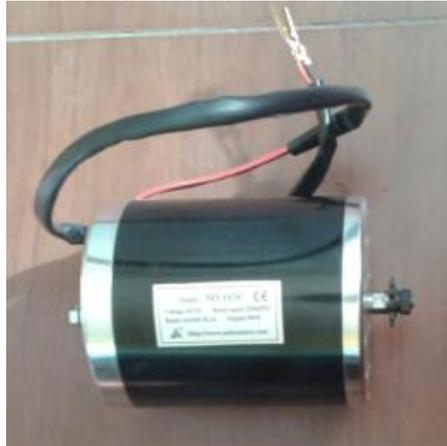
Figura 108 Motor 500W – 36V
