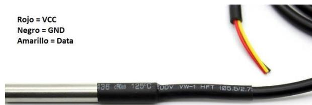
**Figura 26** Dallas temperature sensor ds18b20.
