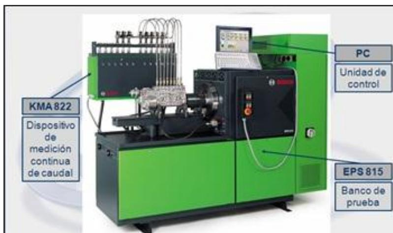
**Figura 22 Partes Bosch EPS 815**
