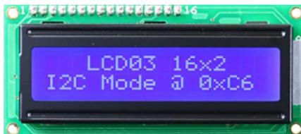
Figura 100 Display lcd 16X2
