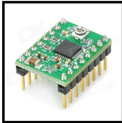
A4988 Stepper Motor Driver
