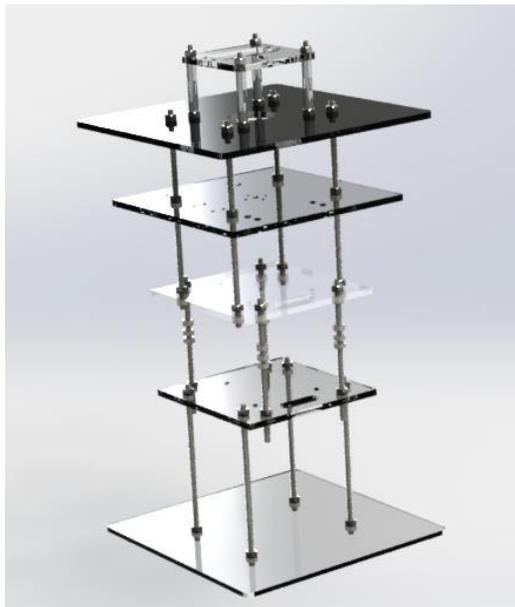
**FIGURA 37. ESTRUCTURA INTERNA**
