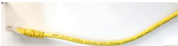
Figura 32 Cable RJ-45 Patchcord
