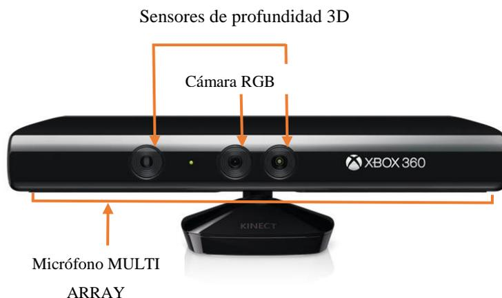
**Figura 13 Sensor Kinect**
