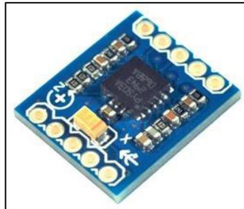
**Figura 35. Giroscopio MEMS**
