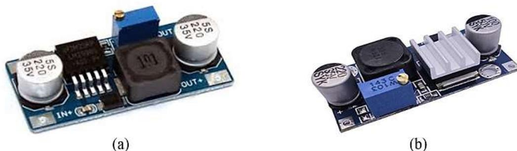
**Figura 42** (a) Convertor DC-DC LM2596S sin disipador, (b) Convertor DC-DC LM2596S con disipador
