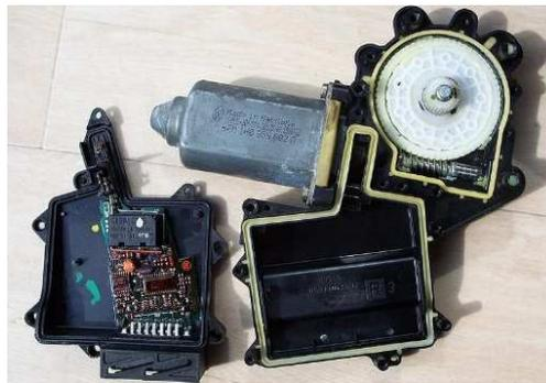
**Figura 32. Motor reductor 12VDC**
