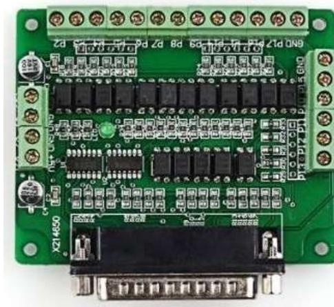
Figura 17.- DB25 breakout board.
