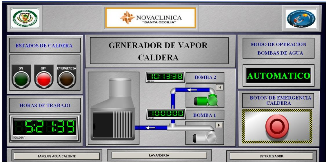
Figura 158. Caldera apagada – HMI.
