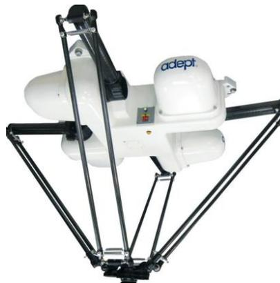
**Figura 18 Robot Paralelo Adept Quattro s650H**
