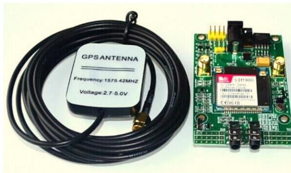
**Figura 53.** Tarjeta SIM908 GSM, GPS, GPRS.
