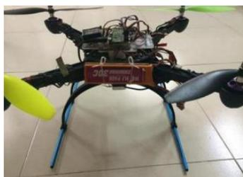
**Figura 3. UAV with NavStik and Odroid**
