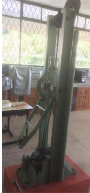
**Figura 61** Máquina: Amsler Pendulum Impact Testing Machine
