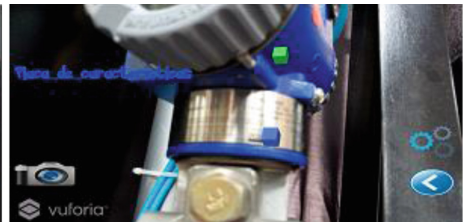
(b) Detection of Rosemount 3051s transmitter parts
