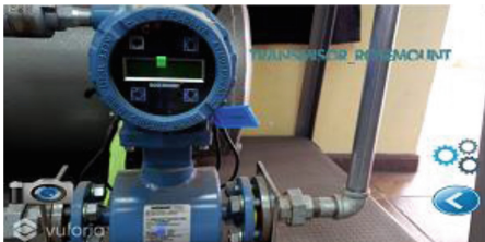
(a) General recognition of Rosemount 3051s transmitter parts
