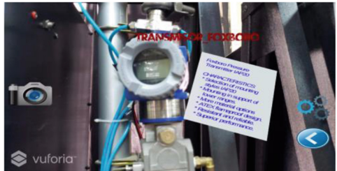
Fig. 5. Use of the application in the pressure station in the Industrial Instrumentation Laboratory.
